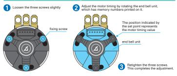
The higher the motor timing, the higher the maximum RPM will be, but at the same time, the more heat will be generated. To prevent breakdowns, make sure that heat generated during 5 to 10 minutes of driving is below a maximum of 70°C.
